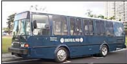
The 30-foot flight crew shuttle bus at Hickam Air Force Base is the first fuel cell vehicle operated by the US Air Force.
